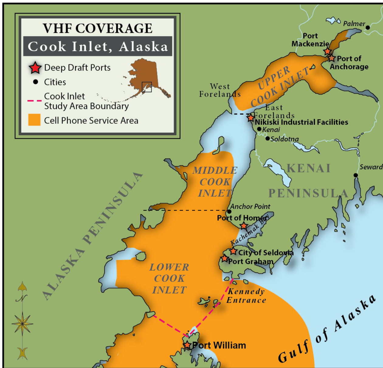
Figure 7. U.S. Coast Guard VHF coverage in Cook Inlet based on a vessel with one watt (based on information provided by USCG Sector Anchorage)
